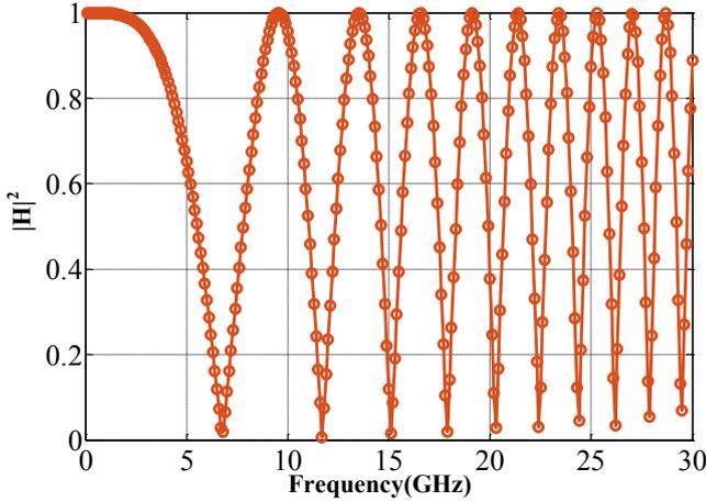
Fig. 1. CD induces serious frequency-selective power fading for IM-DD systems after 80 km transmission.
