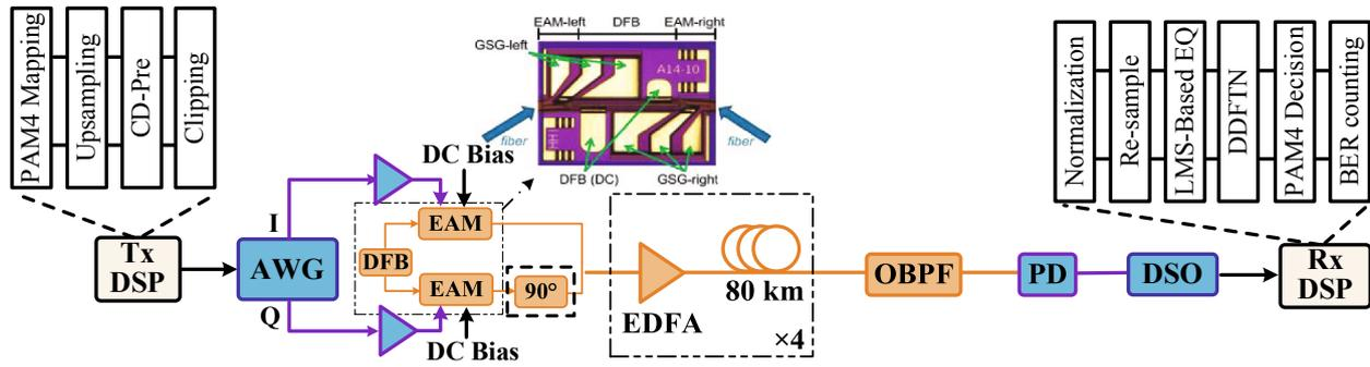
Fig. 3. Simulation setup and corresponding DSP procedures for a 128 Gb/s PAM4 signal transmission using DS-EML quasi-linear modulator.
