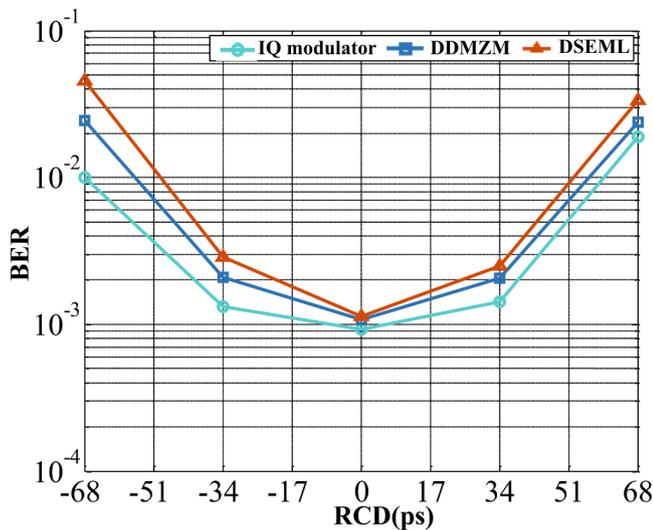
Fig. 6. Simulation results for BER vs. residuals chromatic dispersion (RCD) for a 112 Gb/s CD pre-compensation PAM4 signal with IQ modulator, DDMZM, DS-EML.
