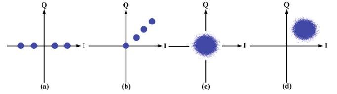
Fig. 2. Operational principle of the proposed transmitter, (a) constellation diagram of the original PAM4 signal (without DC), (b) constellation diagram of the generated PAM4 signal using the proposed transmitter, (c) constellation diagram of the CD pre-compensation PAM4 signal (without DC), (d) constellation diagram of the CD pre-compensation PAM4 signal using the proposed transmitter.
