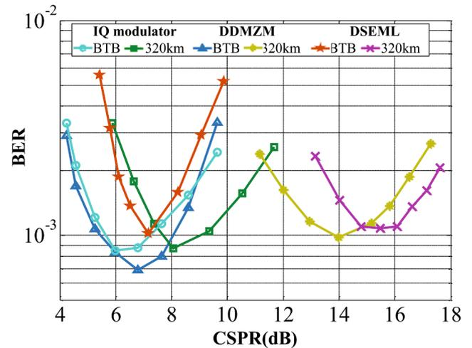
Fig. 5. Simulation results for BER vs. CSPR for a 112 Gb/s CD pre-compensation PAM4 signal with IQ modulator, DDMZM, DS-EML.
