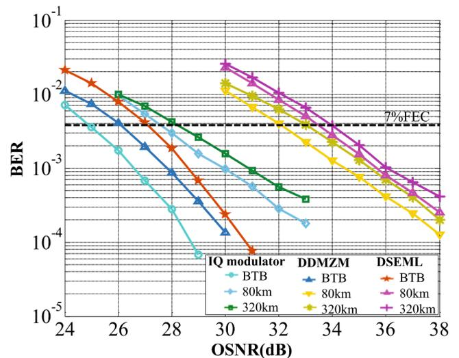
Fig. 7. Simulation results for BER vs. OSNR for a 112 Gb/s CD pre-compensation PAM4 signal at optimal CSPRs with IQ modulator, DDMZM, DS-EML.
