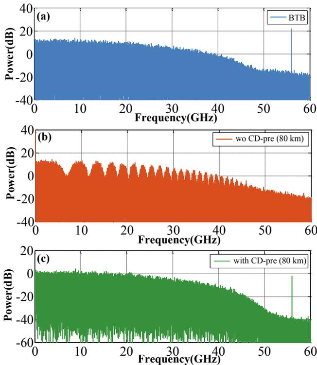
Fig. 4. Electrical spectrum for a 112 Gb/s CD pre-compensation PAM4 signal after PD detection, (a) back to back (BTB) transmission, (b) after 80 km transmission without CD pre-compensation, (c) after 80 km transmission with CD pre-compensation.
