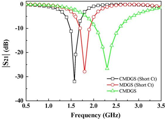
Fig. 5. Simulated transmission coefficients for the CM-DGS resonator with short circuits, M-DGS resonator with short circuits, and CM-DGS resonator.
