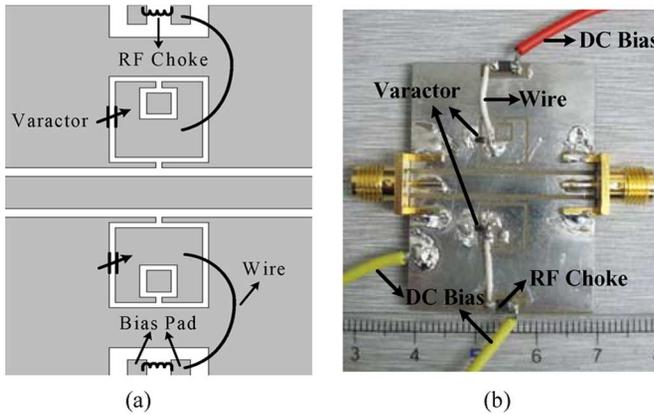
Fig. 6. (a) Schematic layout of the tunable bandstop resonator. (b) Fabricated tunable bandstop resonator.
