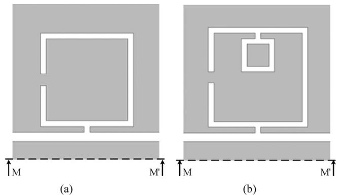
Fig. 4. Layout of the short circuits configuration for (a) M-DGS resonator and (b) CM-DGS resonator (half symmetrical view).
