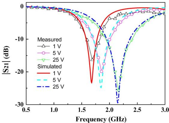
Fig. 7. Simulated and measured transmission coefficients for the tunable bandstop resonator.
