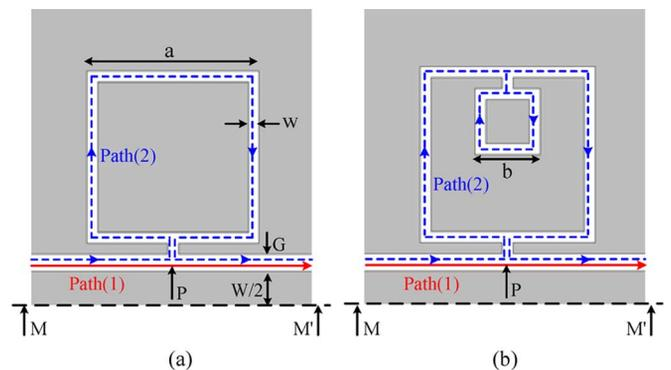
Fig. 1. Schematic diagram of (a) M-DGS resonator and (b) proposed compact M-DGS resonator (half symmetrical view).
