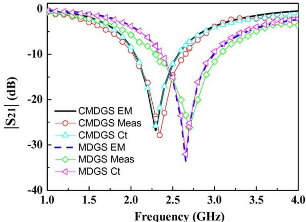
Fig. 2. Electromagnetic (EM) and circuit (Ct) simulated and measured transmission coefficients for the M-DGS and CM-DGS resonator.
