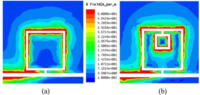
Fig. 3. Magnetic field distribution of (a) the M-DGS resonator at 2.7 GHz and (b) the CM-DGS resonator at 2.3 GHz.
